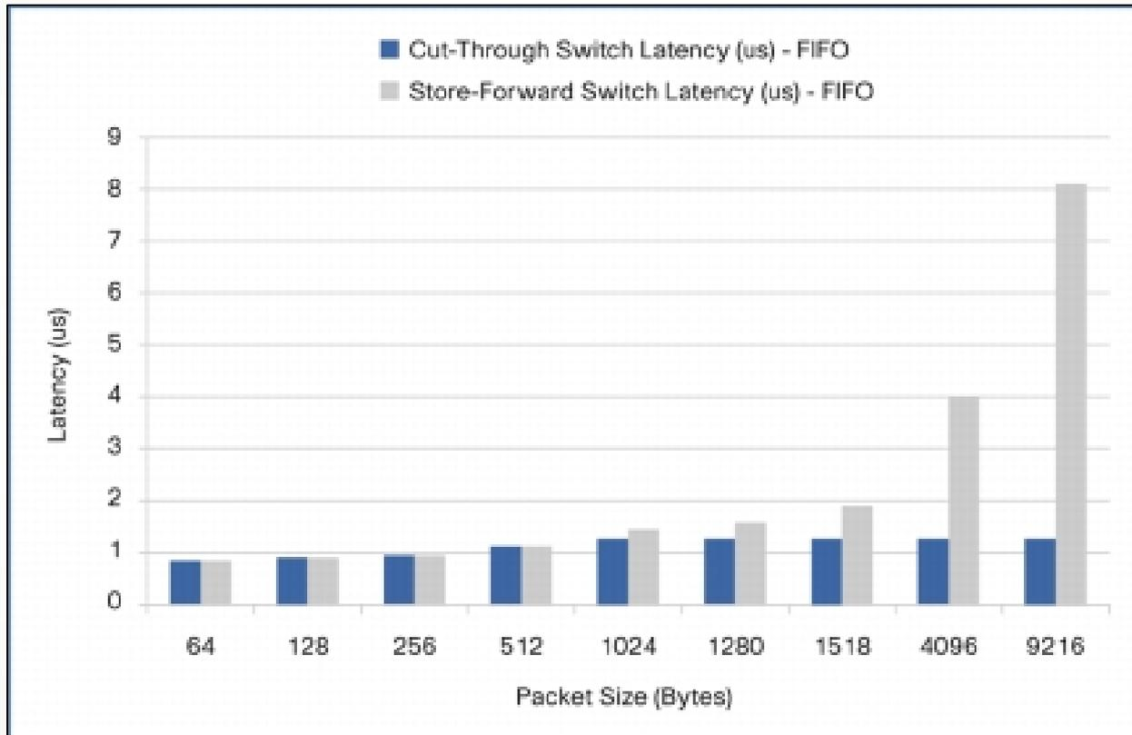
Store-and-forward vs. Cut-Trough using 10 Gb channel
