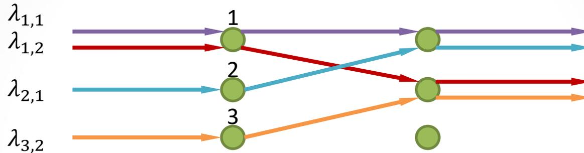
**(A1)** Let the throughput of each communication link be 1, then the flow rates are equal to:
