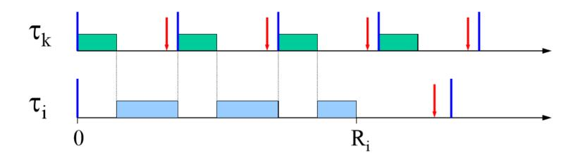
Interference of  $\tau_k$  on  $\tau_i$  in the interval  $[0, R_i]$ :
