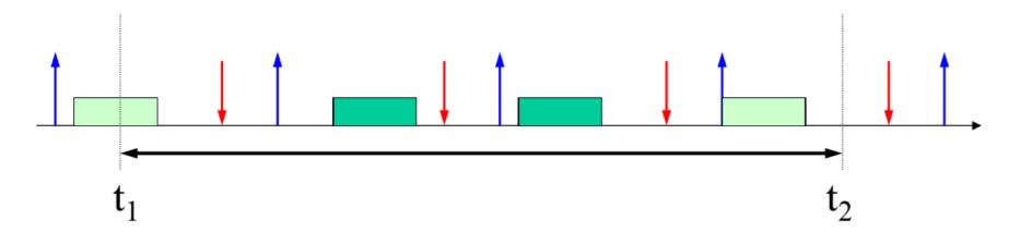
The demand in  $[t_1, t_2]$  is the computation time of those jobs started at or after  $t_1$  with deadline less than or equal to  $t_2$ :
