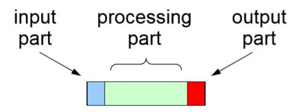
The idea is to force input and output parts to execute in a time-triggered fashion, using timers:
