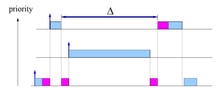
Occurs when a high priority task is blocked by a lower-priority task a for an unbounded interval of time.
